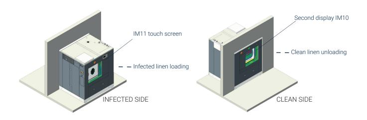
The D2W line is designed and constructed in respect of the EN14065 standard which defines a management system able to provide an appropriate level of microbiological quality according to the use of the fabric and based on the Risk Analysis and Biocontamination Control (RABC) system assessment
